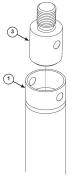
7. Insert the 1/4-20 x 1-1/4" Hex Head Screw (#5) through the aligned holes. Secure with the 1/4-20 Nylock Nut (#4) and firmly tighten.
